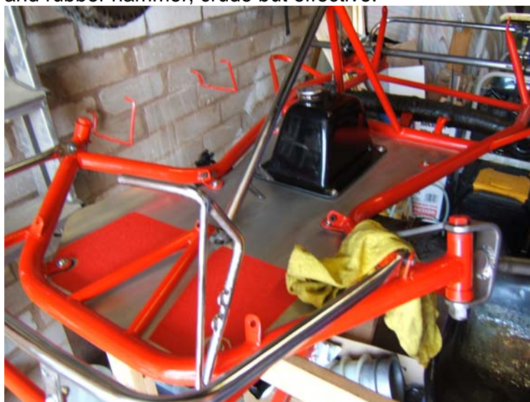
I cut it with an ordinary electric jig saw with HSS blade and bent it carefully with a B&D workmate and rubber hammer, crude but effective.
